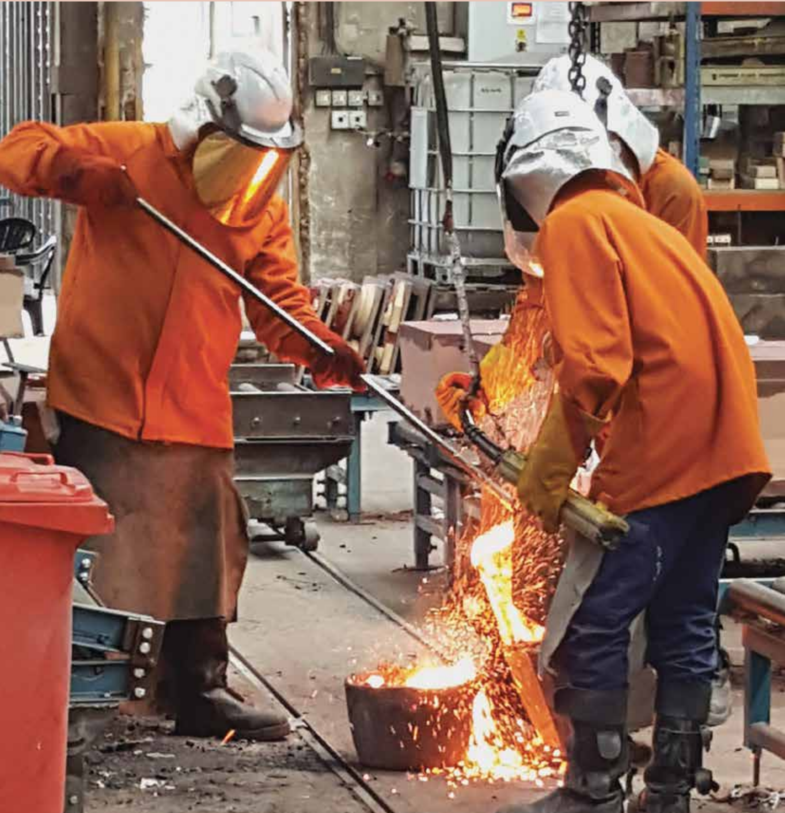
Cast iron work for the new courtyard roof in production at FSE Foundry, Braintree
